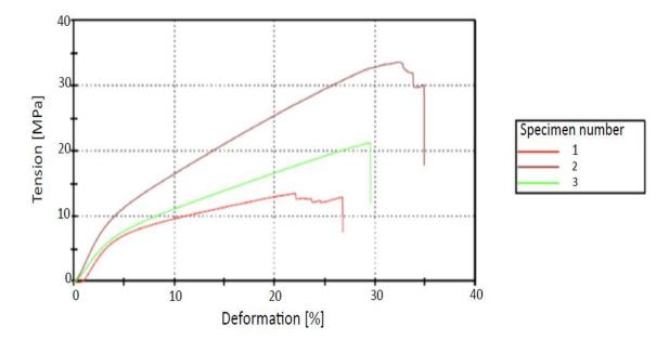
Figure 6: Stress-strain curve of the Jason - Straumann collagen membrane.
