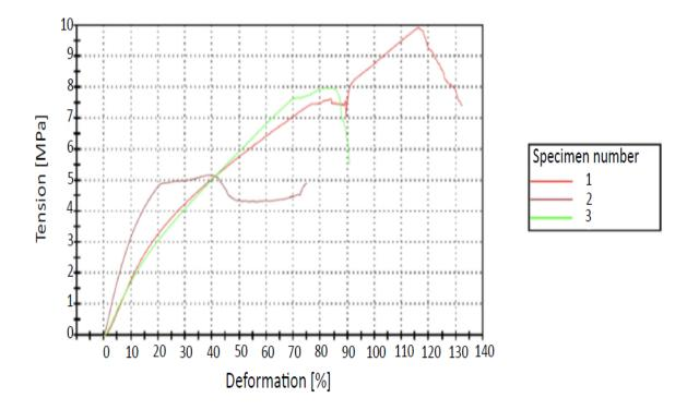
**Figure 5:** Stress–strain curve of Bioguide - Geistlich Pharma collagen membrane.
