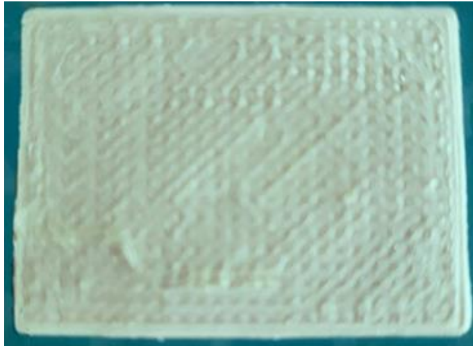
Figure 8: PLA scaffold placed on LUMINA-COAT barrier (3X).
