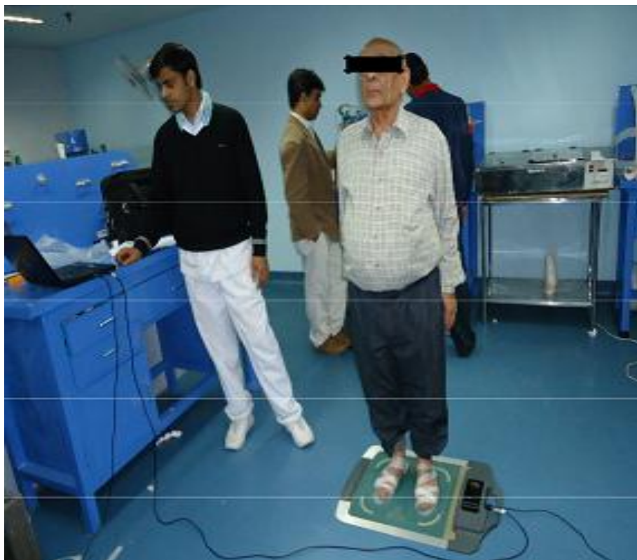
Fig 8: Subject on force plate performing static paedobarographic measurements with insole.
