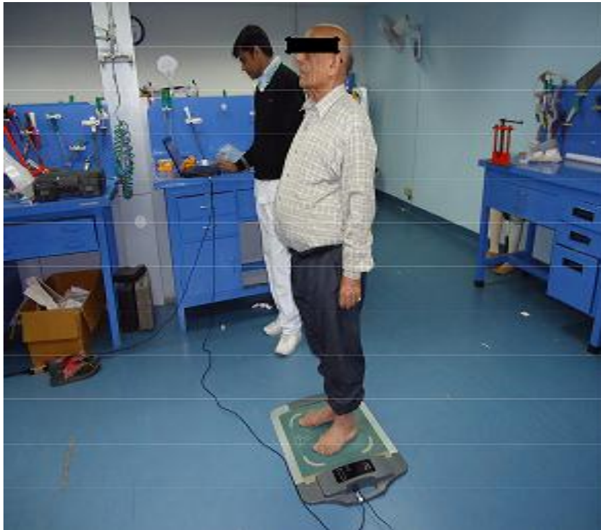
Fig 8: Subject on force plate performing static paedobarographic measurements with insole.
